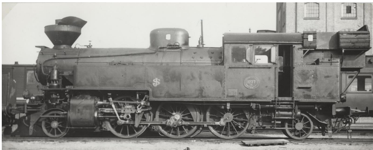
SJ Sa 1277 rebuilt for wood burning. Notice the extensions of the rear buffers to give space for extra wood storage. Photo from the 1940's.
