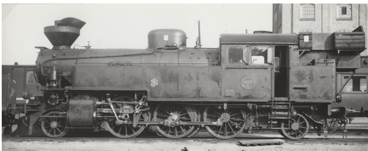
SJ class Sa 1277 rebuilt for burning wood. Photo from the 1940's. Note the extended back buffer plate.
